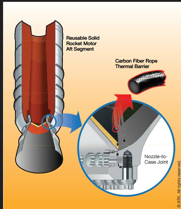
*Using carbon fiber rope instead of rubber insulation in solid rocket motor nozzle joints simplified the joint assembly process and improved shuttle safety margins.*
