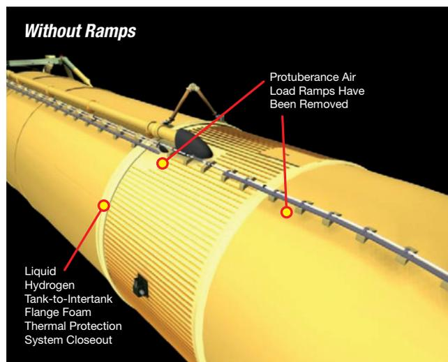
*NASA decided to delete the tank's protuberance air load ramps and implement design changes to the 17 ice frost ramps on the liquid hydrogen tank. Both these measures required adjustments in the components' Thermal Protection System configuration and application processes. Materials and techniques were also altered to improve the Thermal Protection System closeout of the flange joining the liquid hydrogen tank with the intertank.*
