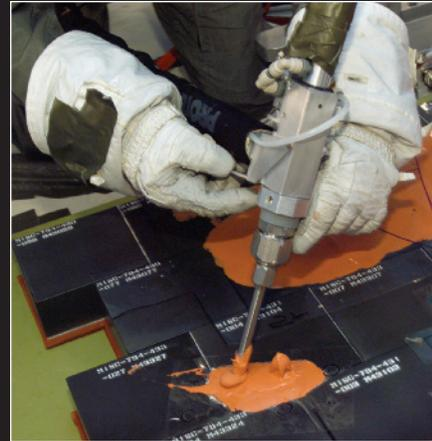
*Ground test of Orbiter tile repair.*
