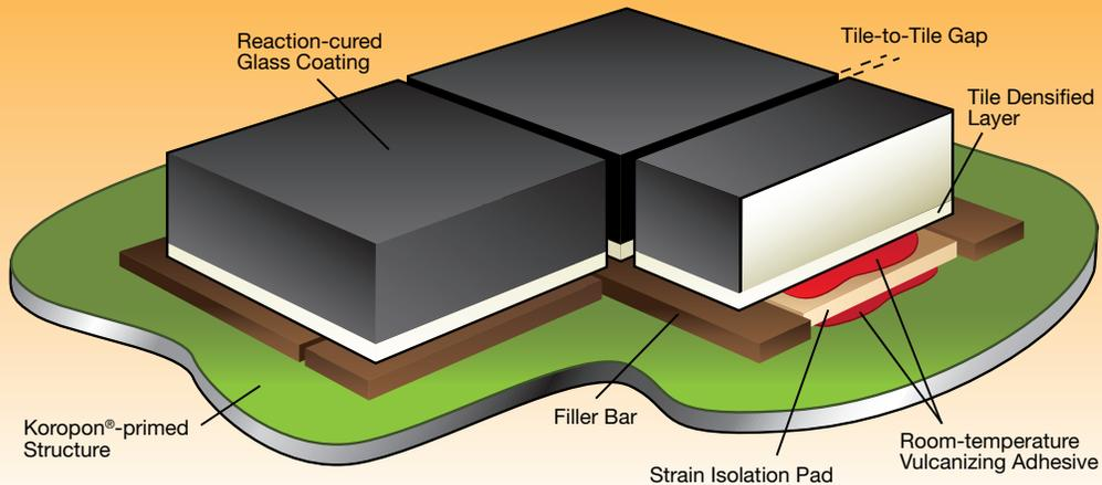
transfer. Selection was based on the temperature on the vehicle. In areas in which temperatures fell below approximately 1,260°C (2,300°F), NASA used rigid silica tiles or fibrous insulation. At temperatures above that point, the agency used reinforced carbon-carbon.
