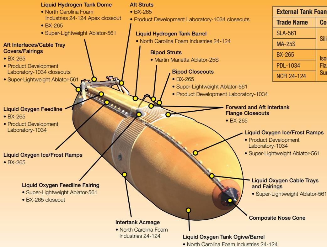
The External Tank's Thermal Protection System consisted of a number of different foam formulations displayed here. NASA selected materials for their insulating properties, and for their ability to withstand ascent aerodynamic forces.
