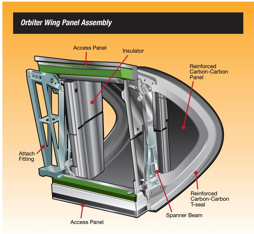
and coating have a different coefficient of thermal expansion. Impregnating the carbon part with tetraethyl orthosilicate and applying a brush-on sealant provides additional protection against oxygen paths to the carbon from the craze cracks.
