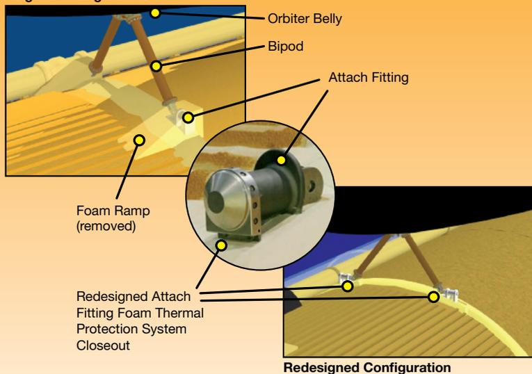
*After the Columbia accident, NASA implemented a number of improvements to External Tank components and related Thermal Protection System elements. One such measure was the redesign of the Orbiter/External Tank attach bipod fitting mechanism, which included a meticulous reworking of the attach fitting Thermal Protection System configuration.*
